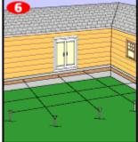
7. The grid formed by the nylon line should be the same as the grid on your plans showing the structural members (girders) which will in turn support the joists, which support the finished deck boards. The intersection of the string lines indicates the center of the post bases.
